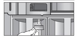
■ Pull the rubber connector down and out.
